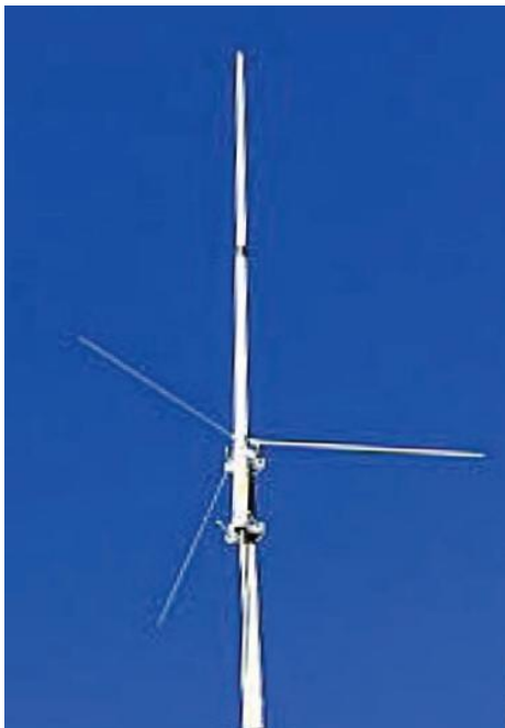
Typical vertical base station antenna
