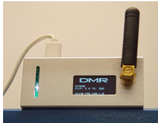
An example of a DMR radio connecting to an internet linked DMR Hot Spot
